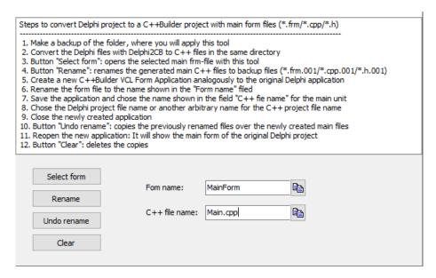
After you have selected the main form of the Delphi application, the name of the form and the name of the according C++ unit are shown in the fields of *MainFormExchange*. As in the previous example the main form is called *MainForm* and the main unit is called *main.cpp* in the picture.
