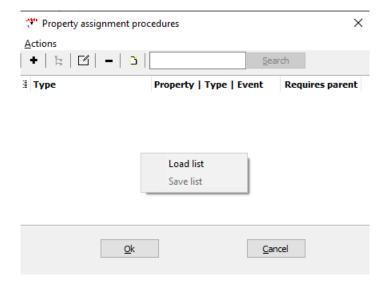
The menu item for loading the file is only enabled if the list of functions is empty.
